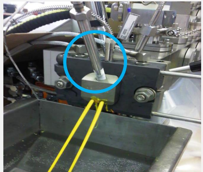
*Fig. 2: RPMP in the extruder die-plate*
