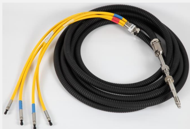
Figure 1: Combined UV-VIS + NIR probe for reflectance and/or transmission application. Hastelloy probe tip with sapphire window. Probe design with \frac{1}{2} "-20UNF (typ. Dynisco®) made for 200 bar and 350 °C
