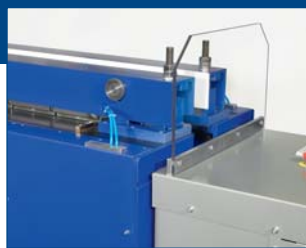
Lower position of the height adjustable clamping beams
