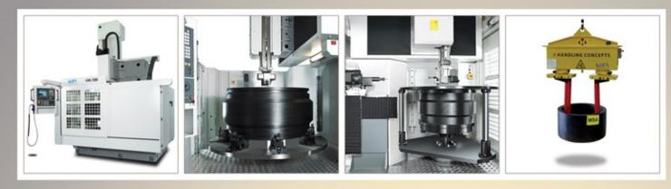
The VWL 710 and VWL 1200 are vertical format, 3-axis, CNC controlled electrofusion wire laying machines, designed for the wire laying of medium to large fittings or pipe sections. The machines are equipped with software dedicated to producing fittings in the range 125 to 900mm internal diameter (VWL 710), and 125 to 1400mm internal diameter (VWL 1200).
