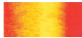
Thermoscan of a PE-coating film without Promix Melt Blender
