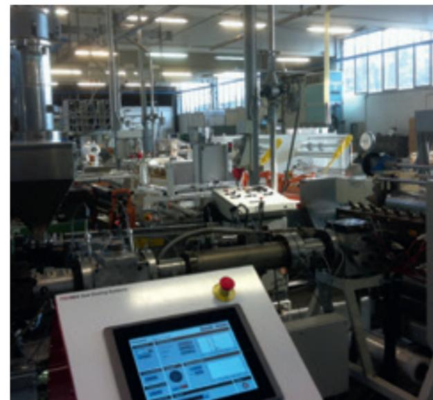
Promix N2 Dosing System as part of a foam extrusion line
