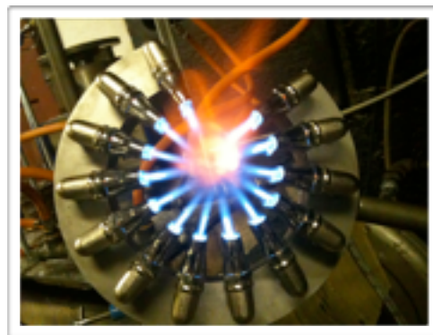
Circular high intensity burners for surface melting and adjustment prior to stretching
