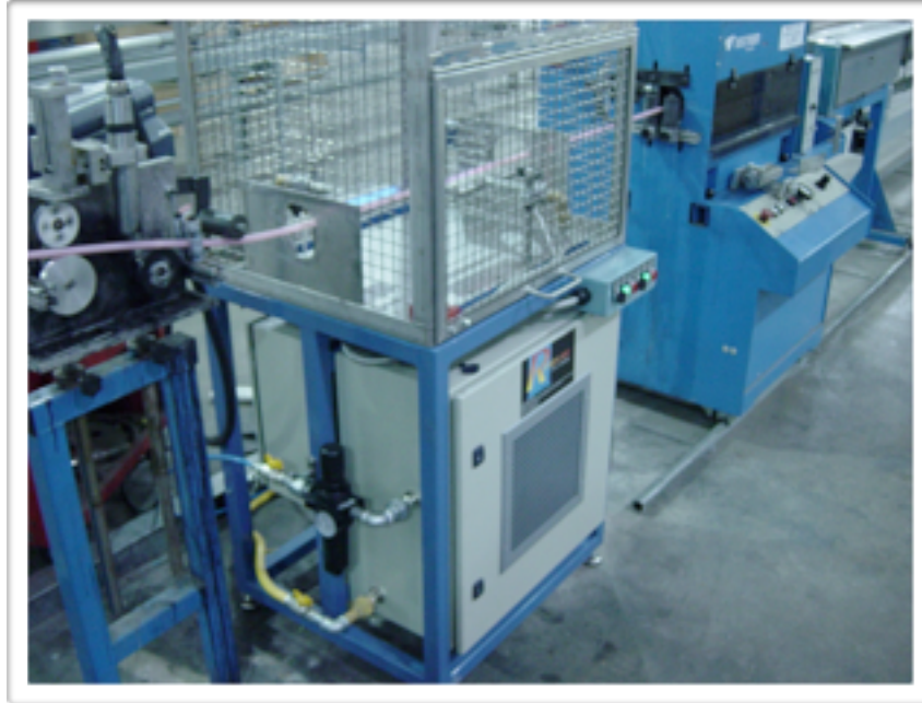
Packed system on plastic tube extrusion lines
