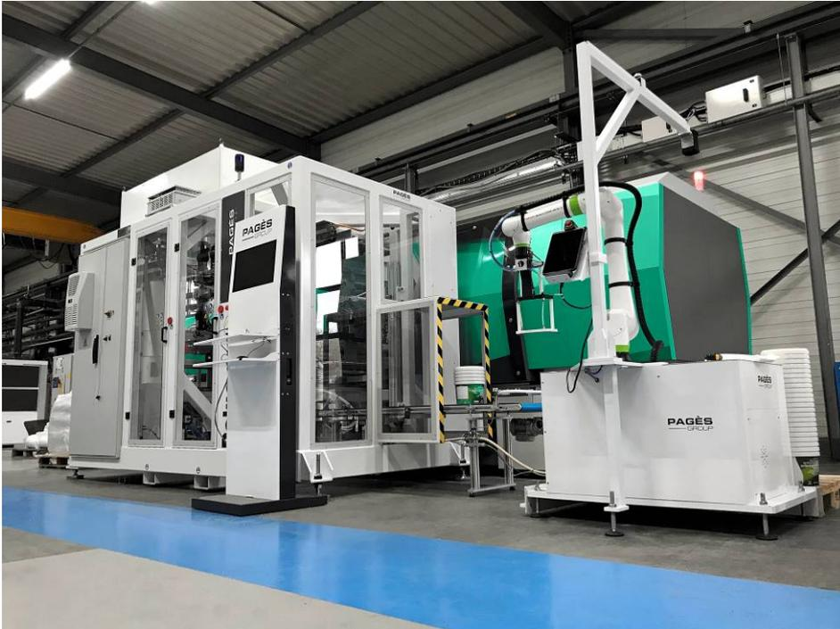
*Fully automated injection moulding cell around a hybrid Allrounder 720 H in packaging version.*
