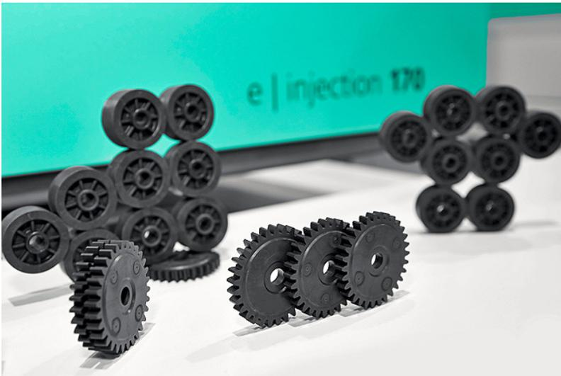
*Plastic-bonded magnetic material: At the FIP 2022, an electric Allrounder 470 A will alternately produce a magnetised toothed wheel and a pole wheel.*
